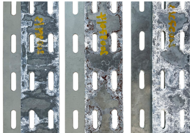
ZM - Continuous galvanizing with magnesium and aluminum admixture S - Pre-Galvanized F - Hot Dip Galvanized
