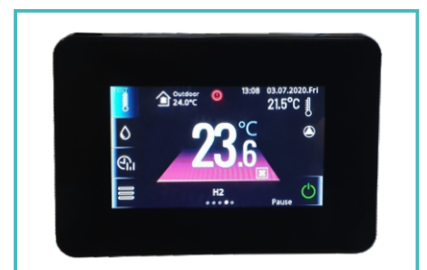
Control panel with a color touch screen
