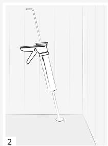
2 Injection of the chemical anchor into the hole
