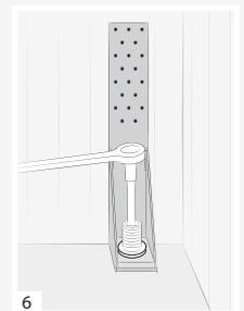
6 Positioning of the nut by adequate tightening
