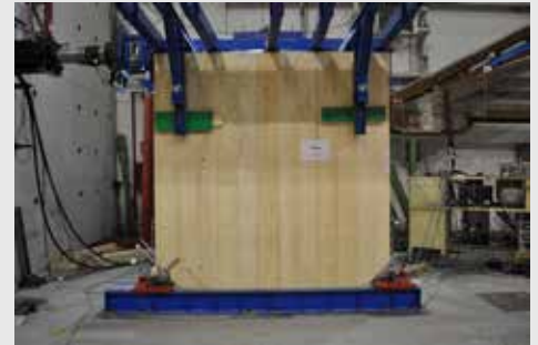
Example of output from cyclical test on wall system: force-displacement diagram and test setup for single panel
