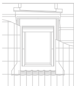
recessed installation - concrete roof
