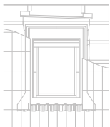
recessed installation above rafter insulation
