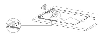
F Seal cleaned cut-out edge with silicon, fill
