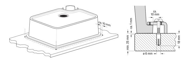
For a precise fit, the cut-out must be produced in the worktop by reference to the original sink. The supplied installation templates provide guidance here.
