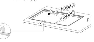
**H** Remove any excess silicon.
