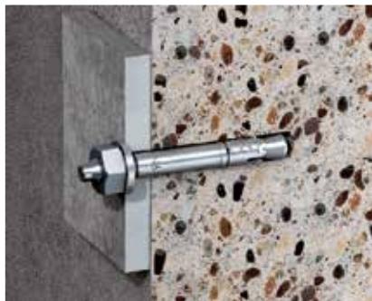
Nail tie, type N, with threaded connection Nail tie, type N, with M6 threaded connection, usable in cracked or non-cracked standard concrete C20/25 to C50/60.
