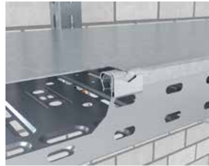
Screwless cover mounting Screwless cover mounting takes place with unperforated covers and the cover clamps, type DK DRLU. The cover clamp is simply fixed in the rail of the cable tray.
