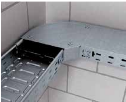
Mounting of fitting cover The fitting cover is fastened to the cable tray using turn buckles; this is done by clamping the turn buckle under the rolled up side rail of the cable tray with a 90° turn.
