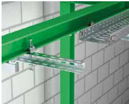
Cantilever beam on steel Mounting of U support as cantilever beam on steel girder. Fastening with clamping angles or chuck jaws depending on load. Fastening with spacers, type DSK.
