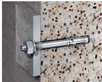
Bolt tie, type BZ Bolt tie, type BZ, for fastening heavy-duty anchorings in cracked or non-cracked standard concrete C20/25 to C50/60, suitable for push-through mounting, with M8, M10, M12 or M16 thread.
