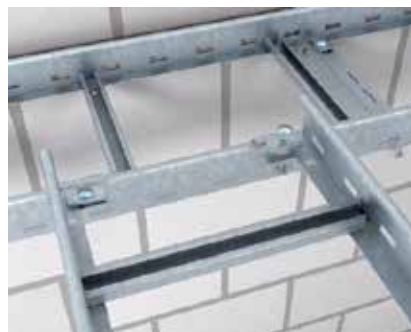
Mounting of a T exit Creation of a horizontal T exit of two cable ladders at different heights. The support profile, type LAW, is required to fix two cable ladders.
