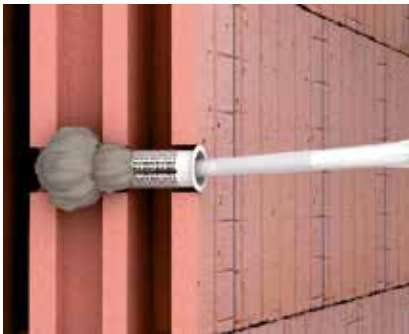
Applying the injection mortar Press in the injection mortar from the cartridge from the base of the drill hole to the opening. In so doing, draw the point back slowly.
