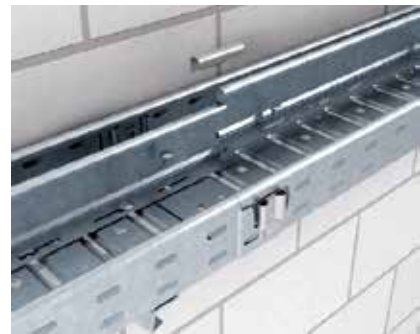
Screwless barrier strip mounting Screwless barrier strip fastening of the barrier strip TSG 60, with truss-head bolts M 6x12. The barrier strip can simply be run over the joint and connected without bolts using the barrier strip connector TSGV.
