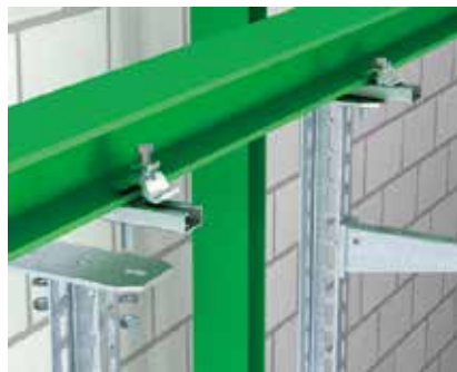
Clamp fastening with additional C profile Use of an additional C profile rail, type MS, for wider steel girders. Route along steel girder.
