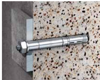
High-load anchor, type SZ High-load anchor, type SZ, with M12 thread connection for fastening components with high loads, approved for cracked and non-cracked standard concrete C20/25 to C50/60.
