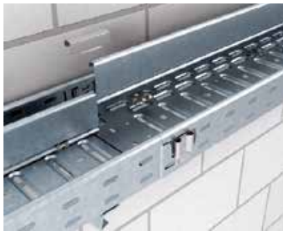
Screwless barrier strip mounting Screwless mounting of the TSG ... barrier strip with the KS KR hold-down clamp. The barrier strip can be run over the joint and connected without bolts and without processing using the barrier strip connector TSGV.
