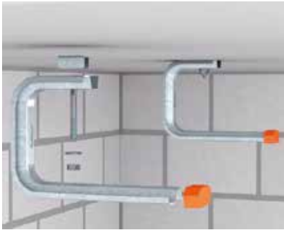
Ceiling mounting of TP wall and ceiling clamp Universal mounting of the TPD wall and ceiling clamp on the ceiling (with DS 4 spacer). Maximum tray width 300 mm.
