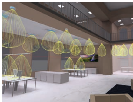
3D view of balanced positioning of sensors and light sources to achieve the desired light distribution.
