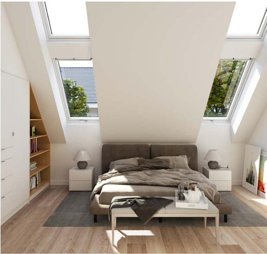
optical enlargement of the space by opening into the truss / larger volume of air / ventilation through the stack effect
