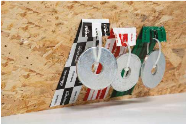
Test campaign on the cohesion and adhesion performance of acrylic adhesive tapes on different substrates.
