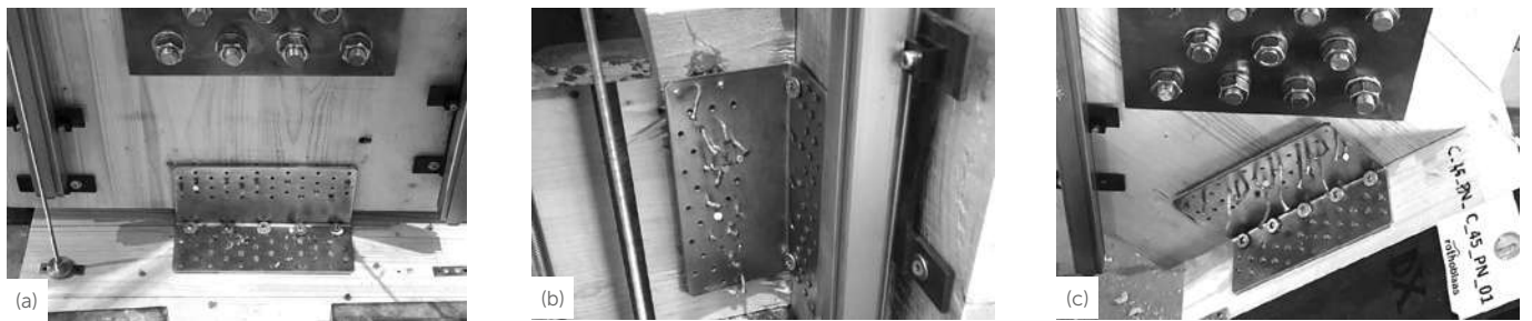
Figure 2. Samples at the end of cyclic tests: tension (a), shear (b) and 45° (c) (partial fastening).
