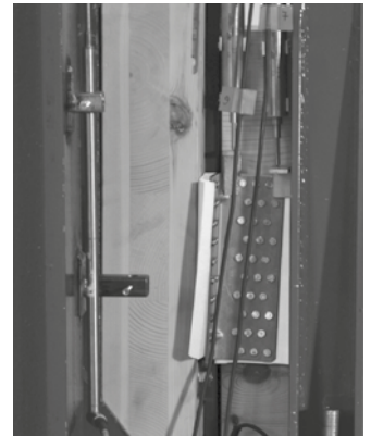
Test samples: CLT panels TITAN TTF200 angle bracket
