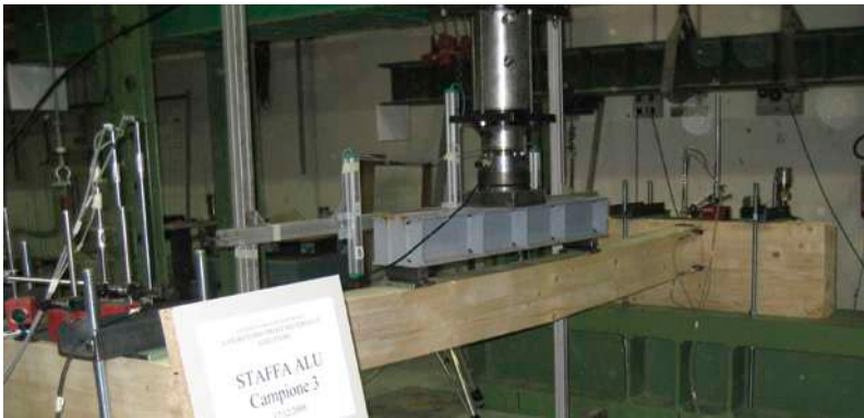
Tests on full-scale specimens (main-secondary beam connection).
