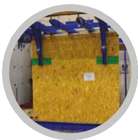
Frame wall during testing
