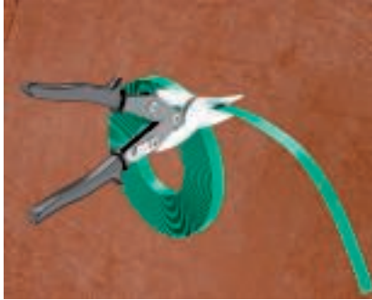
Cutting the tightening strap to size Cut the tightening strap to the required length (e.g. using metal cutters).
